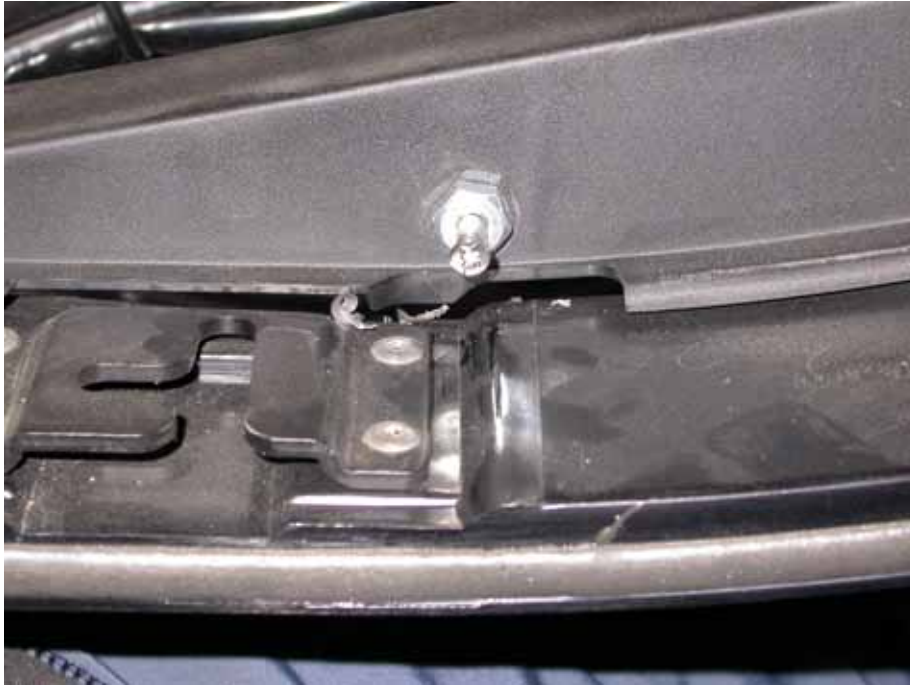
Figure 18. Pin switch installed
