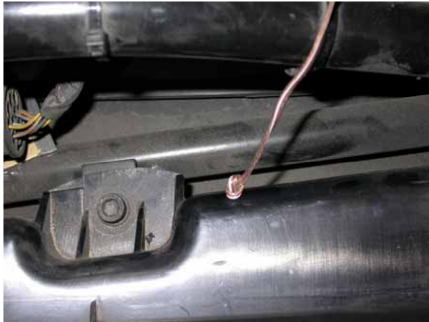
Figure 14. Knot tied in wire so it can't slip back into saddlebag
