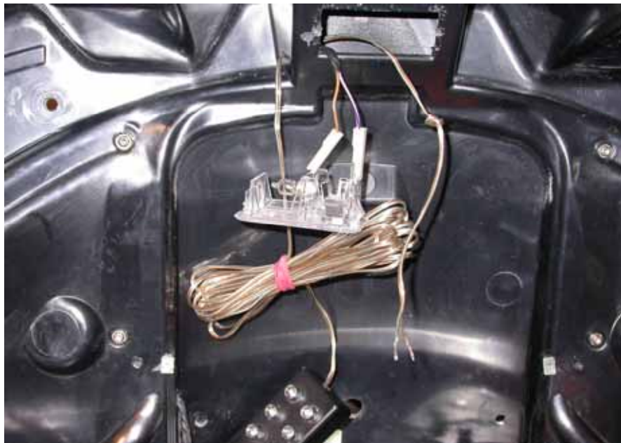
Figure 3: Wire pulled through hole and BMW trunk light opening
