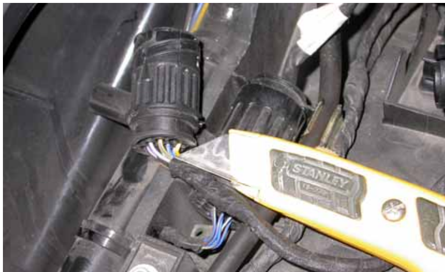
Figure 11. Carefully cut the wrapping with a sharp knife
