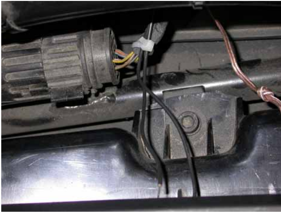
Figure 20. Pin switch wires secured to wiring harness
