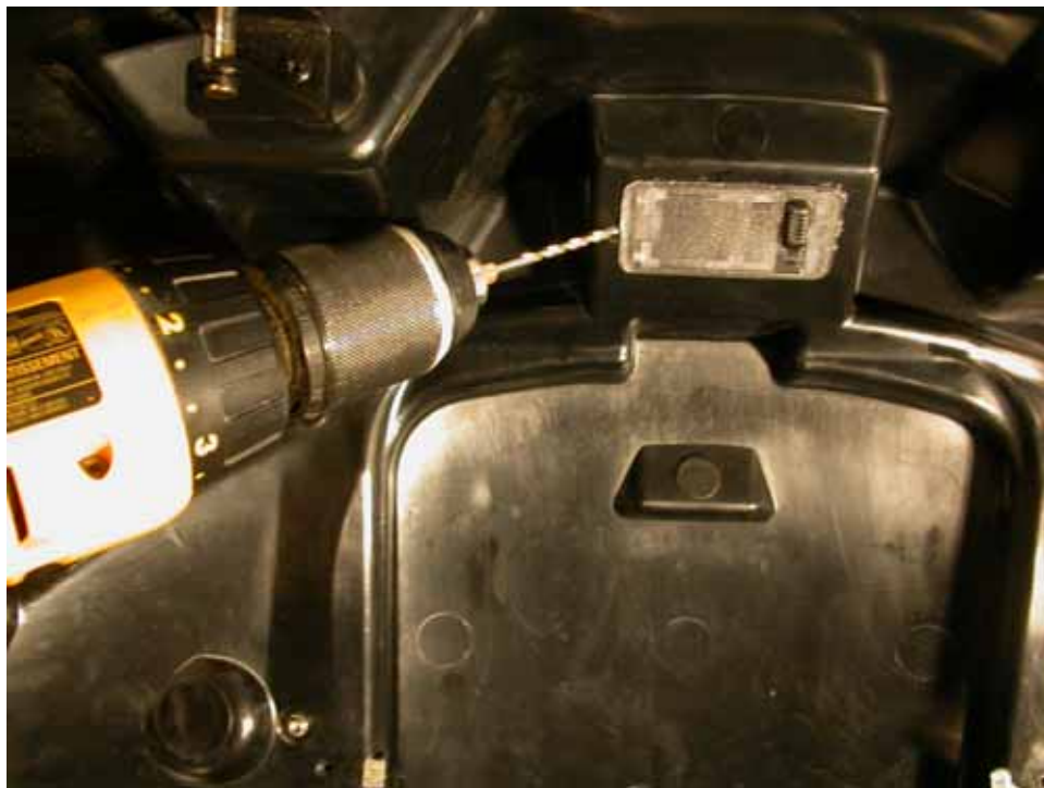
Figure 1: Drilling the release hole
