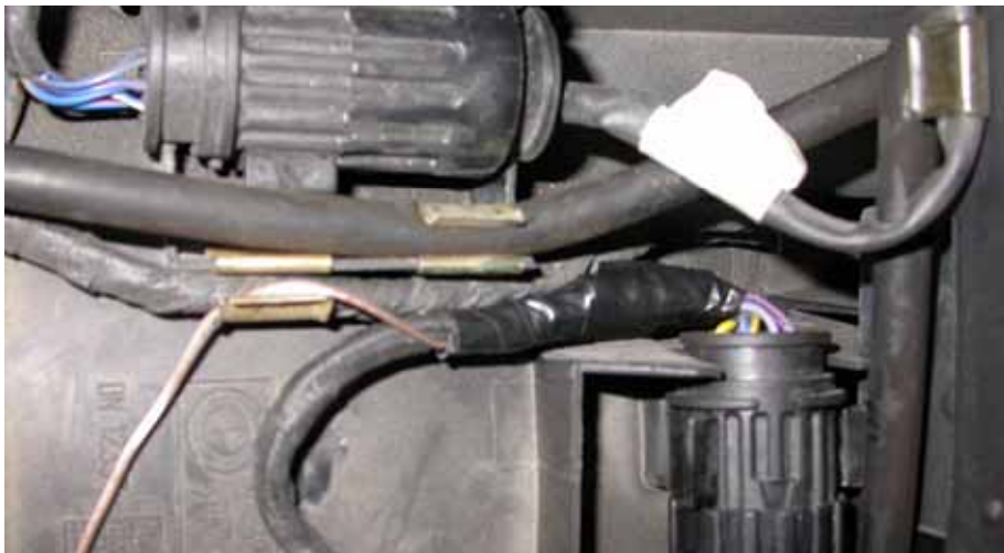
Figure 16. Bundle of wires taped after installing blue butt connector (viewed straight down from left side of bike)
