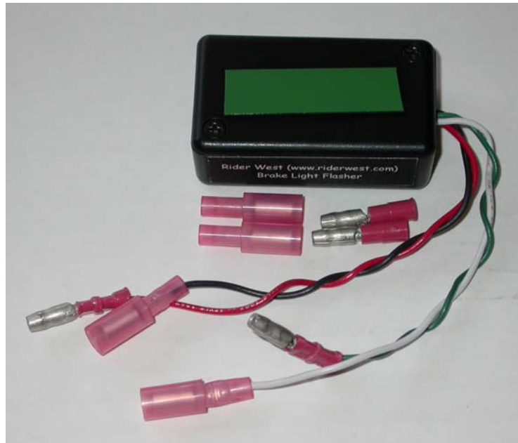
Figure 1. Brake light flasher for center brake light
