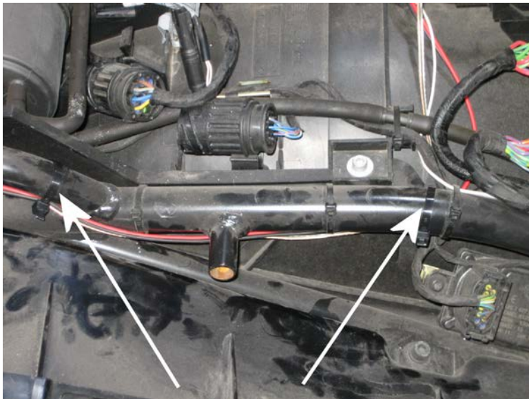
Figure 14. Secure the wires to the bottom of the frame tubing with cable ties.
