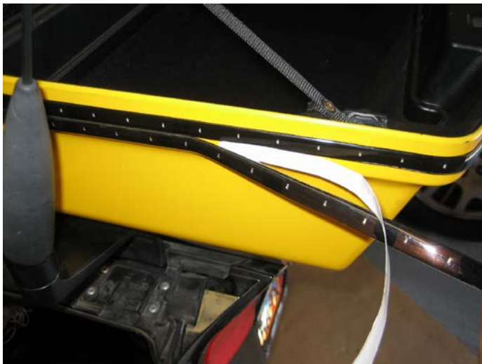
Figure 29. Attaching the left turn signal LED strip.
