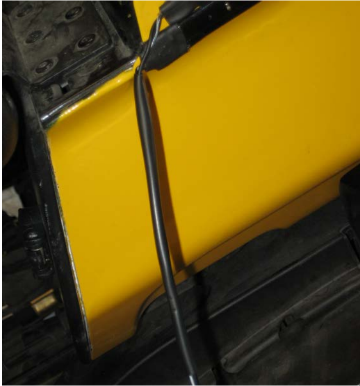
Figure 32. Adding the protective tubing to the wires.
