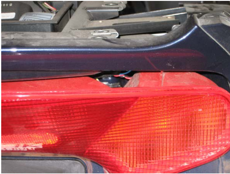
Figure 11: Determining where to drill the hole for the wires.
