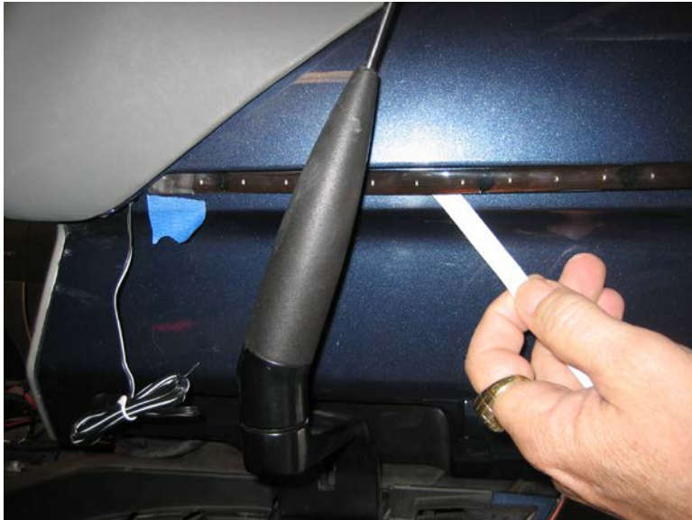
Figure 22. Applying the upper LED strip.
