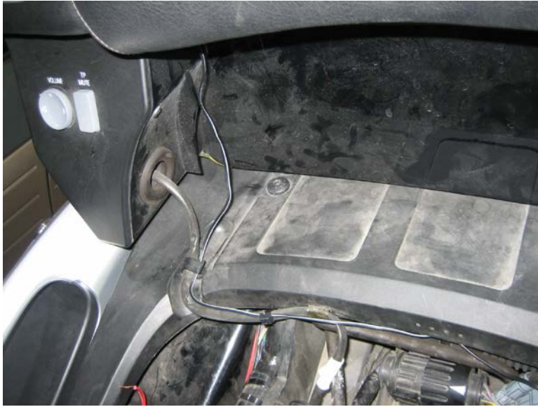
Figure 33. Routing the wire for the right-side LED strip.
