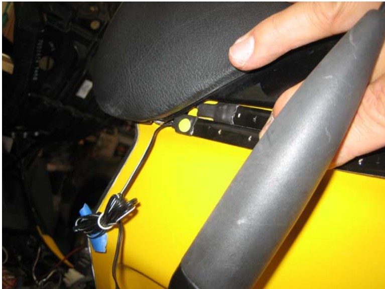
Figure 27. Positioning the left turn signal LED strip.
