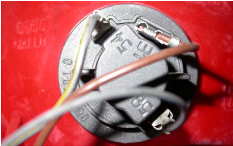
Figure 16: Taillight socket terminal numbers.
