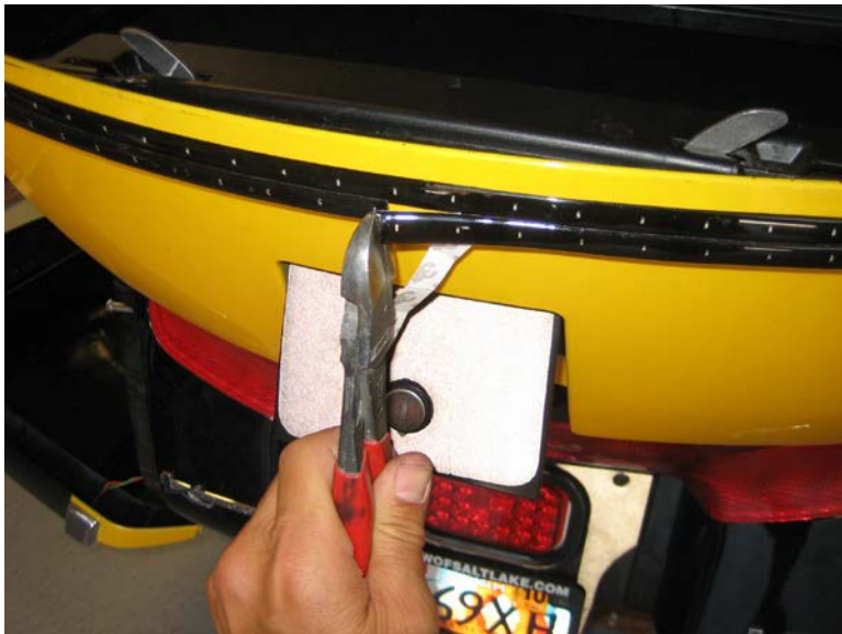
Figure 31. Trimming the right-side LED strip.
