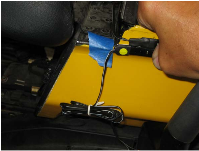
Figure 28. Marking the starting position for the left turn signal LED strip.
