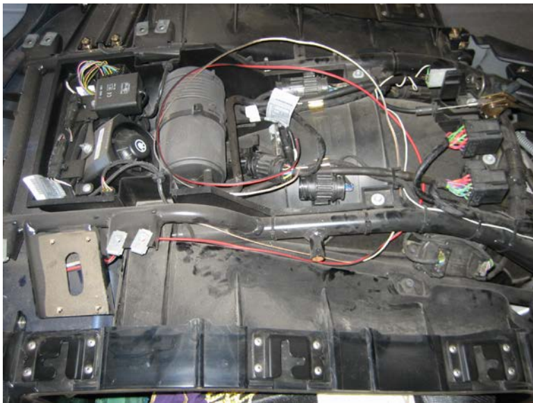
Figure 12: Routing wires from taillight area to under the passenger seat.
