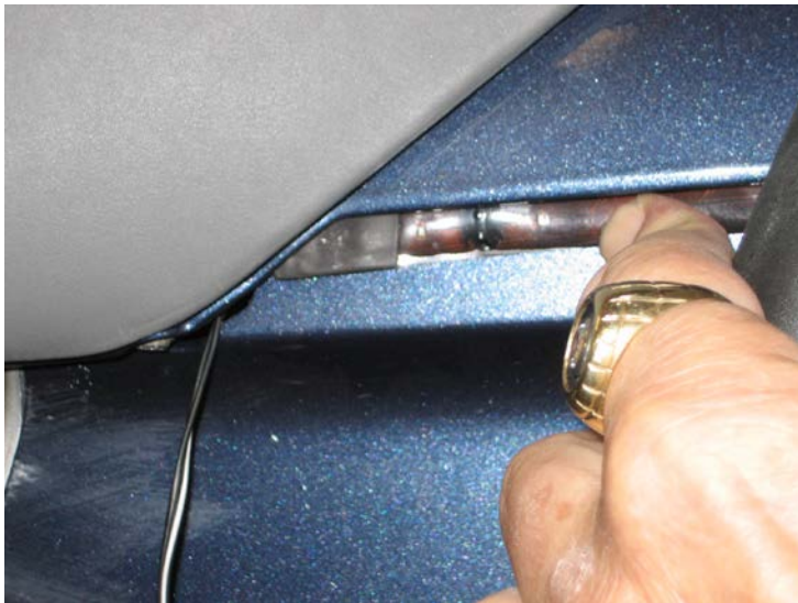
Figure 20. Locating the starting point for the upper LED strip.
