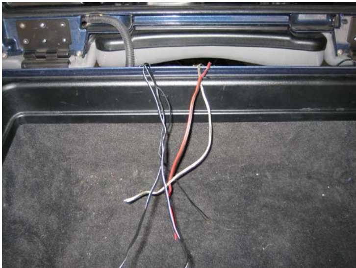
Figure 35. Bring the wires into the trunk so it's easy to work on them.
