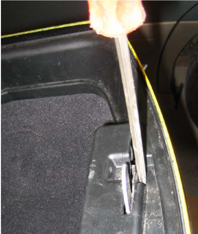
Figure 5: Releasing the tabs holding the trunk liner in.
