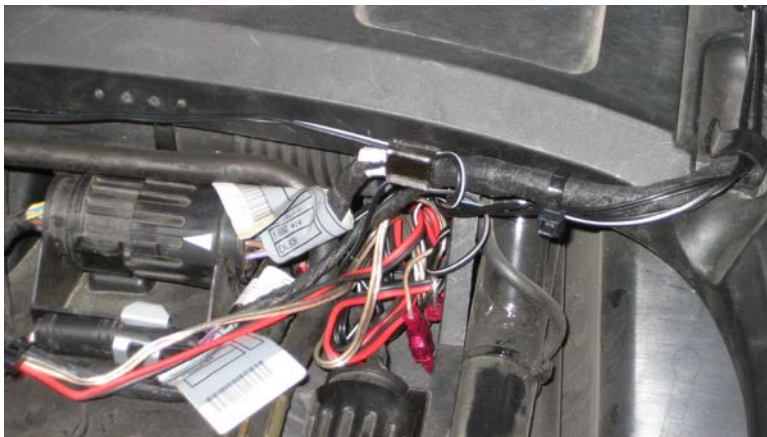
Figure 38. Routing the zip wires under the passenger seat.
