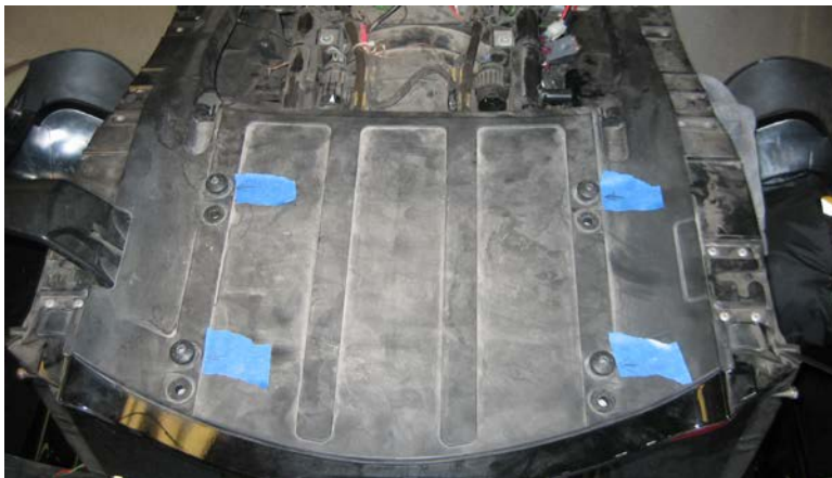
Figure 6: Holes marked with tape on panel under trunk.
