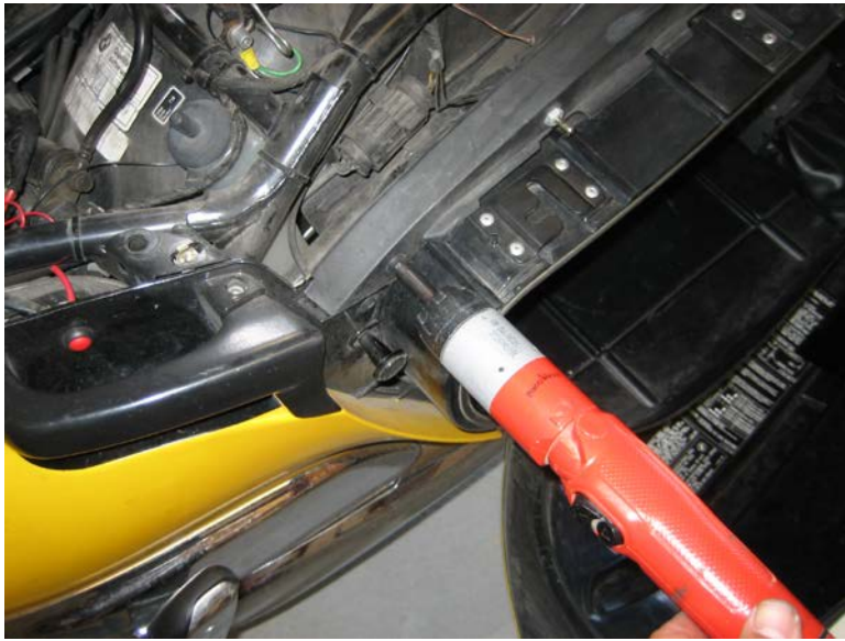
Figure 7: Location of front Torx screws in panel under trunk (left side of bike).
