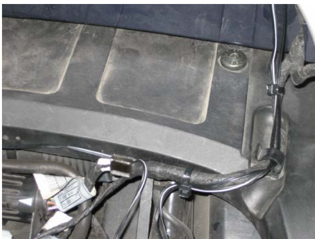
Figure 34. Routing and securing the wire from the right and left LED strips.
