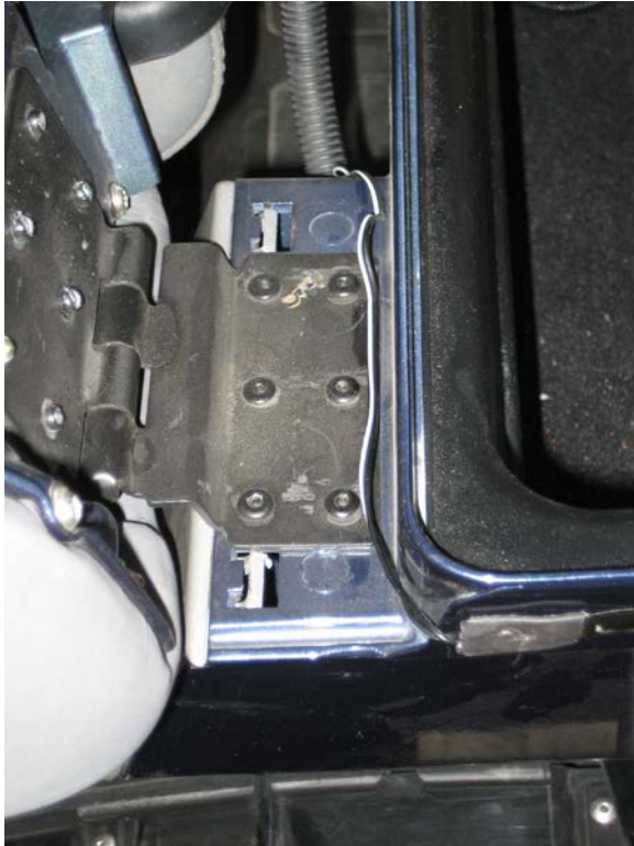
Figure 24. Lay the wire across the hinge to keep it out of the way. Note that the wires in the photos are black and black with white stripe while your wires are clear and clear with red stripe.
