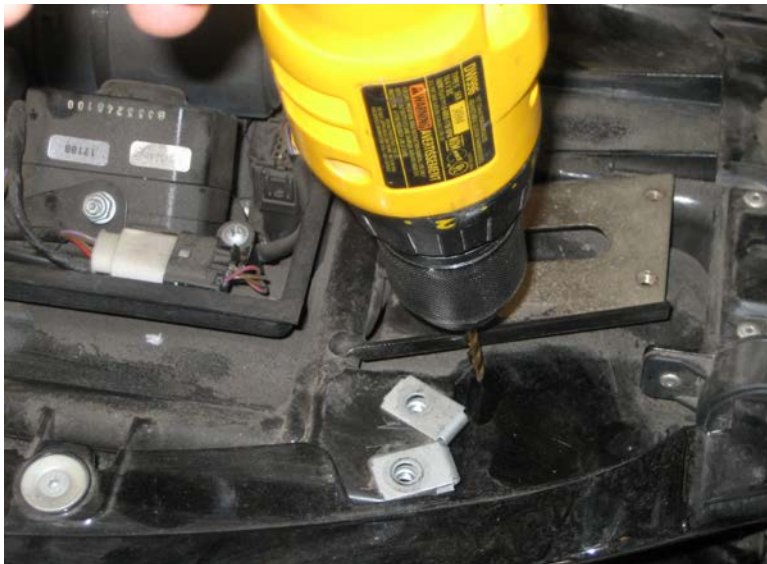
Figure 10: Determining where to drill the hole for the wires.
