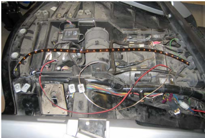
Figure 19. Using one of the amber LED strips to test the wires.
