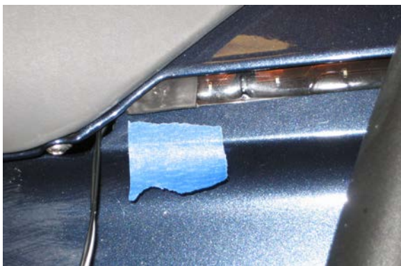
Figure 21. Marking the starting point for the upper LED strip with tape.
