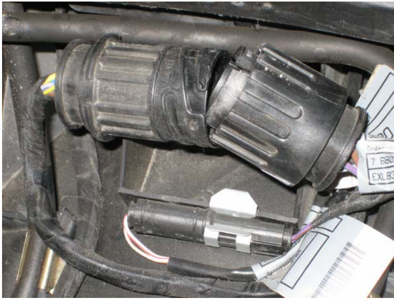
Figure 3: Third connector for 2005 or later model LTs (it's the small connector below the larger one).
