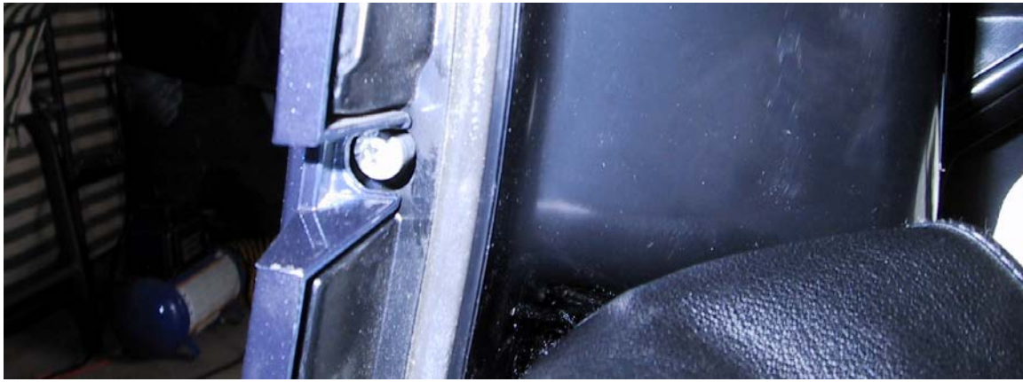
Figure 9. Taillight assembly bolt for 2005 and later LTs (5mm Allen wrench).
