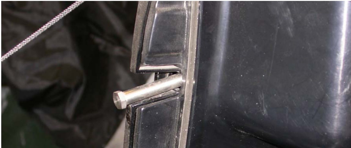
Figure 8: Taillight assembly bolt for 2004 and earlier LTs (10mm socket).
