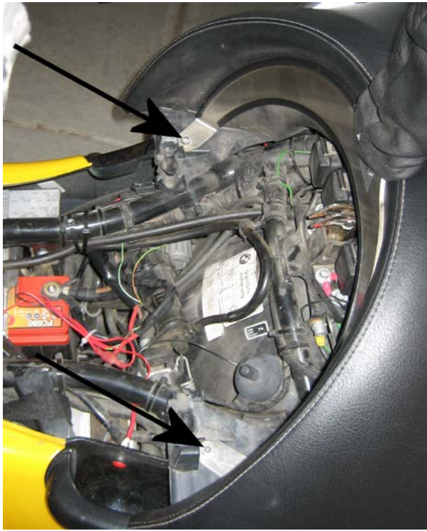
Figure 1: Bolts holding on passenger seat (and back rest on this bike).
